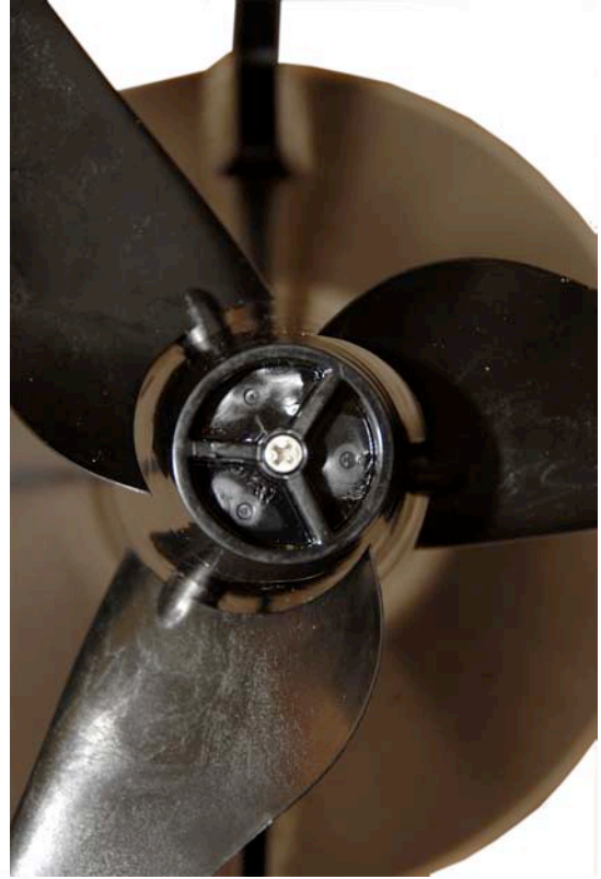
Image 2: Optimum Thrust Top of blade from hub 1/8 " / 3.0 mm
